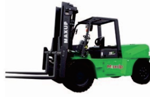
E Series Lithium CPD50/60/70 Rated Load:5000/6000/7000kg Battery:96V/600Ah Lifting height:3000-6000mm
