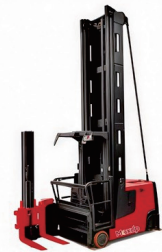
Man-up 3-way Stacker MCC16 Rated Load:1600kg Battery:Lead-acid 80V/560Ah Lifting height:4500-9500mm
