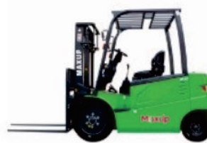
N Series Lithium LG30/35B Rated Load:3000/3500kg Battery:80V/280Ah Lifting height:3000-6000mm
