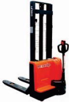
Electric Stacker PSL15/20 Rated Load:1500/2000kg Battery:Lead-acid 48V/40Ah Lifting height:1600-3500mm
