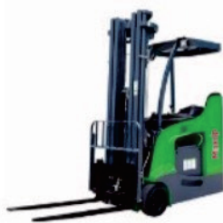
N Series Counterbalance Lead-acid MN18 Rated Load:1800kg Battery:48V/460Ah Lifting height:3000-6000mm
