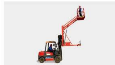
Forklift Manned Lifting Platform
